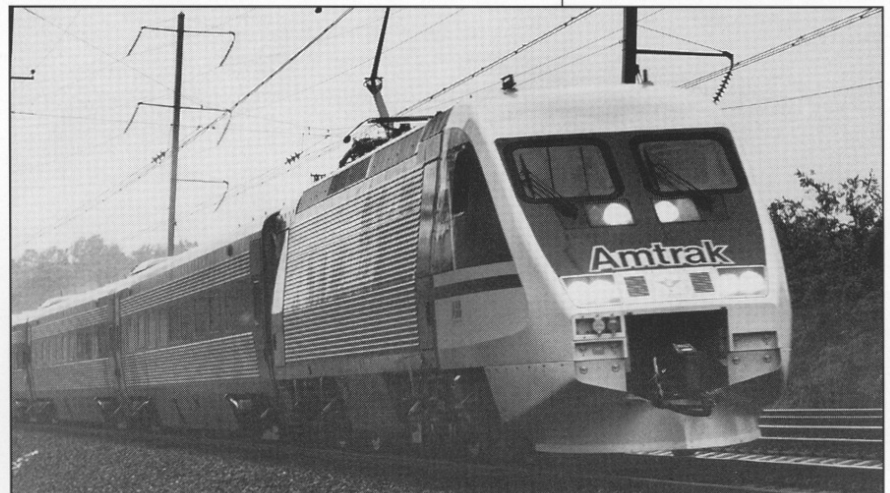
The X2000 demonstrated its "tilt" technology to take curves faster.
