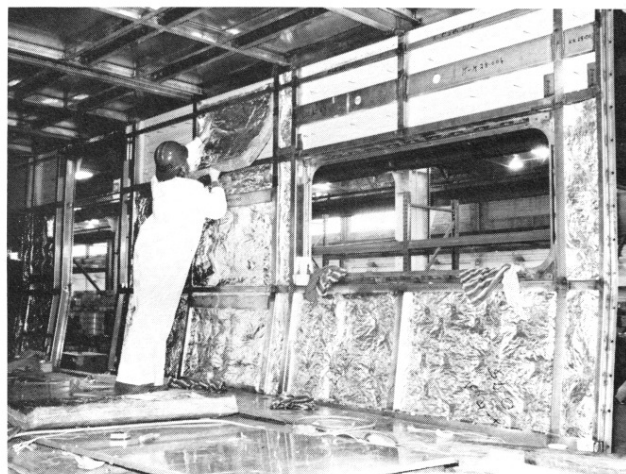
(Left) Welder works on the underside of a new bi-level car. The car rests temporarily on PS shop trucks. (Above) Pullman Standard employee installs insulation, for heat retention and sound deadening, on the PS assembly line.
