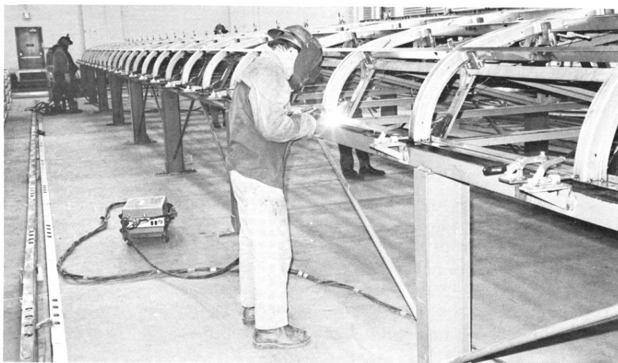
One of Pullman Standard's workers assembles sections that will make up the roof portion of one of Amtrak's new bi-level cars.
