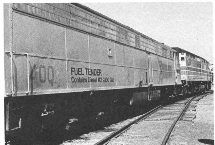
Amtrak's prototype fuel tender was converted from a diesel locomotive. Fuel tanks are located inside the body shell.
