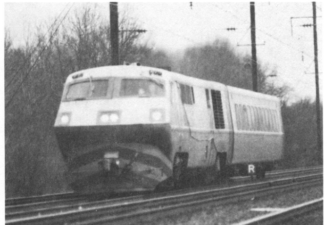
Prototype LRC (for Light, Rapid, Comfortable) train undergoes testing in the Northeast Corridor. Tests proved successful and two LRC train sets have been leased for use in the Pacific Northwest.
